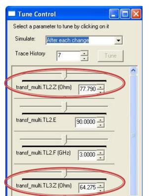
Permanently check that the 5 impedance values are either increasing or decreasing. The 3 transmission line values you tune must be in the correct order and inside the interval imposed by Z<sub>S</sub> and Z<sub>L</sub>
