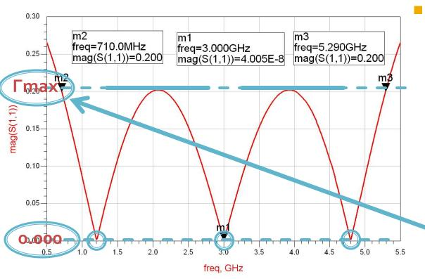
for the Chebyshev transformer the graph is pointed and reaches o.o (or at least o.ooX) at fo and at least two other frequencies and the ripple inside the bandwidth reaches **Tmax** (from your individual subject)
