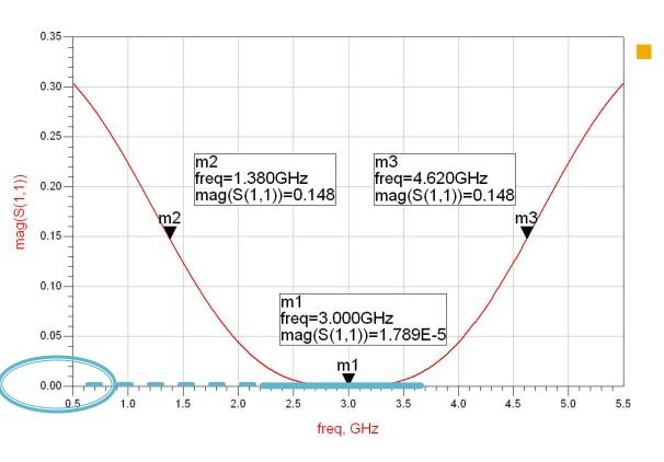
for the binomial transformer the graph must not be pointed/angled in fo but the tangent must be horizontal and reach o.o (or at least o.ooX)
