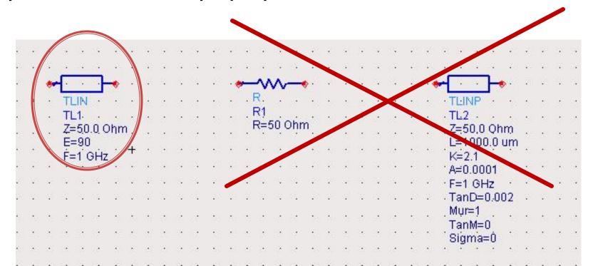
Putting in the schematic instead of terminators/ports (TERM –Simulation Sparam palette) R\_model or even R (Lumped Components palette)
